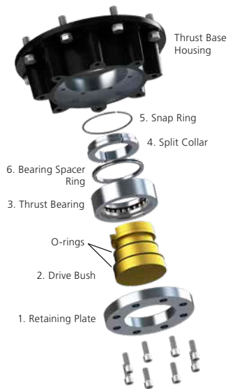
Fig. 5.1.4 F25 & F30 base assembly
