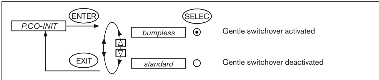
Fig. 83: Operating structure P.CO INIT
